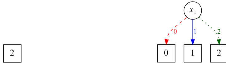
Fig. 3.12 Simple decision diagrams representing a constant function (left) and an integer function of a single variable (right)
